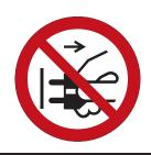
To prohibit unintended disconnection while circuit is live and under load
