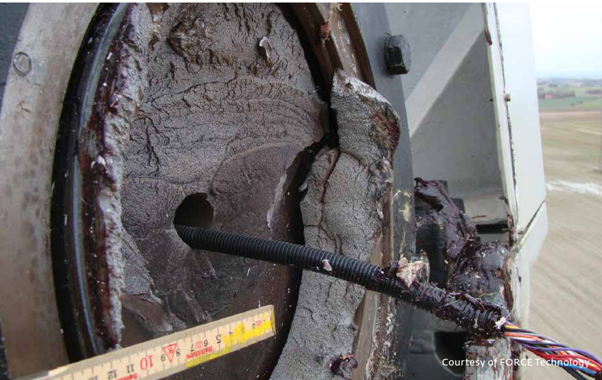
Inspection of broken wind turbine shaft
